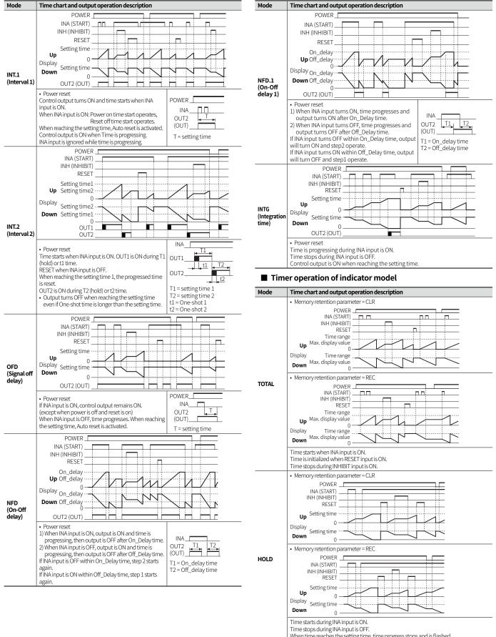
When time reaches the setting time, time progress stops and is flashed. When RESET input is ON, progressed time is initialized.
