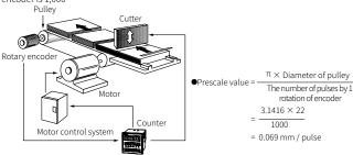
Select decimal point. .-. prescale decimal point: ---. and set prescale value: 0.069. it is available to control conveyor position by 0.1 mm unit.
