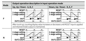
After count-up, counting display value and retained (hold) output are maintained until RESET input is applied.
