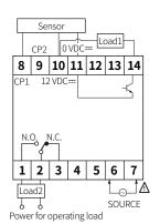
The sum of operating current capacity of load1 and sensor should not be over external power capacity (50 mA).
