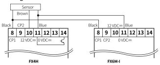
Please connect as the power of sensor is supplied from only one of counters and design input logic with same way.
