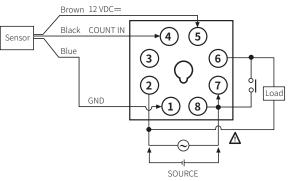
The capacity of sensor power supply is  $12\,\text{VDC}$  =  $50\,\text{mA}$ . Be careful not to exceed the capacity when connecting the sensor. Be careful not to let the load capacity exceed the contact capacity.
